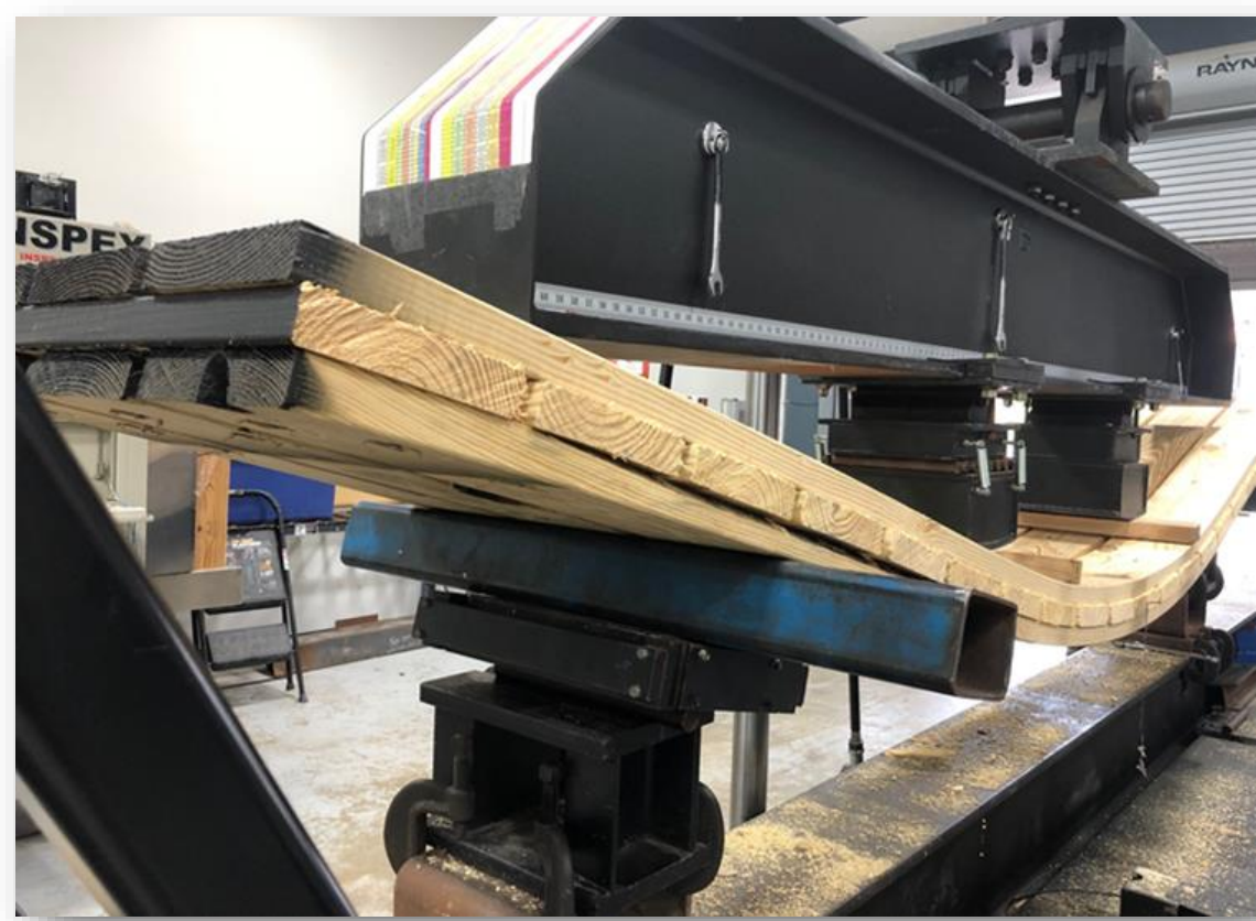
Three-ply solid flexural specimen in the universal testing machine while undergoing a third-point destructive bending test.
