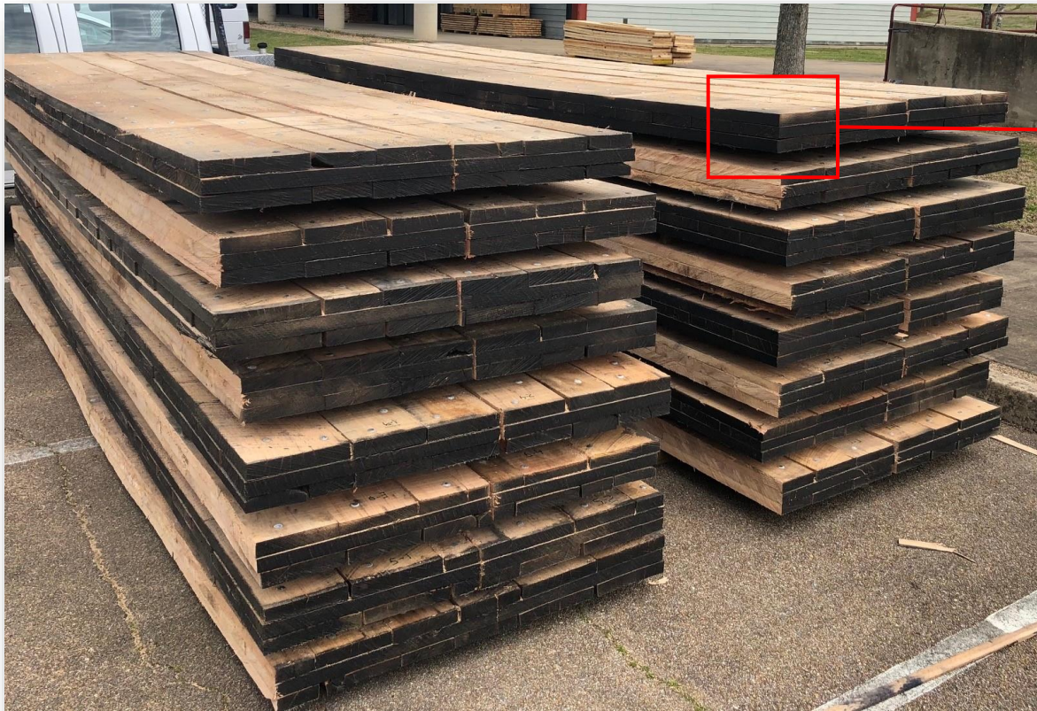
Stack of 32 three-ply solid mat flexural specimens (mixed oak) prepped for testing.
